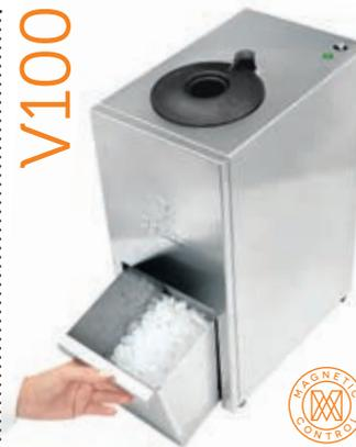
The high-performance commercial ice crusher. The all-stainless steel V100 can crush 6kg ice in one minute, putting it at the top of its category. It is designed to work in all safety for the operator thanks to the double automatic shutoff system, which activates upon lifting the lid or upon removing the crushed ice tray.
